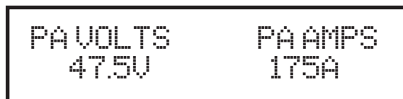
Figure 3-4. Press the FUNCTION Key to read Voltage and Current
