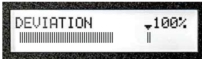
Figure 3-13. Press the FUNCTION Key to read Deviation
